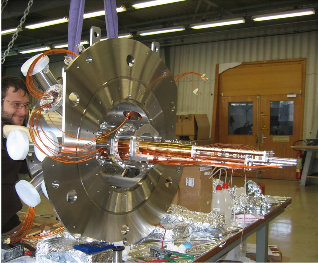
Figure 9 – In picture trap system of the “central region” of the experiment. Trap is mechanically supported by the inner flange that separates Ultra High Vacuum region ( 10^{-10} mbar at 4K) with intermediate region ( 10^{-7} mbar at 70 K)
