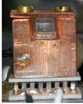
Figure 5-14: Photograph of a severely degraded BBO crystal installed inside the thermalizing copper box. The active thermal element is a small Peltier cell placed below the copper element.
