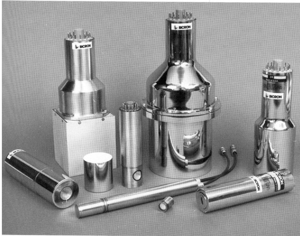
Commercial NaI(Tl) detectors: Integral lines. (Harshaw)
