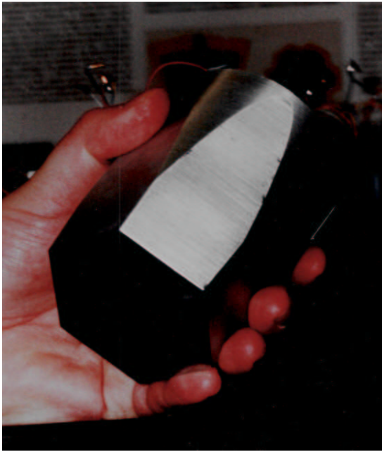
Figure 10.8: The encapsulated Ge crystal for the EUROBALL Cluster detector.
