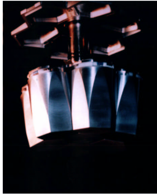
Figure 10.9: Encapsulated Ge crystals arranged in the 7 detector cluster.
