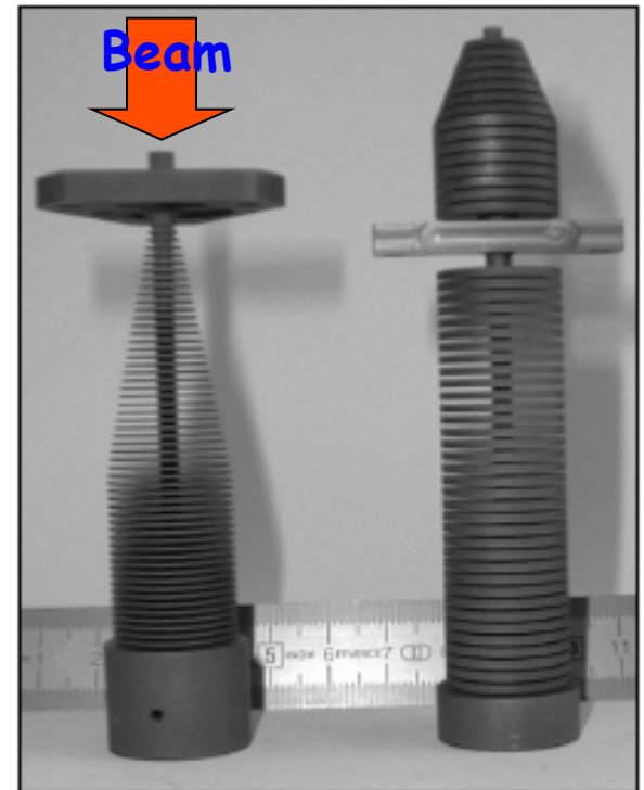
Figure 4 : Picture of the carbon targets : (left) the target dedicated to Ar and Ne production; (right) the target dedicated to He production.
