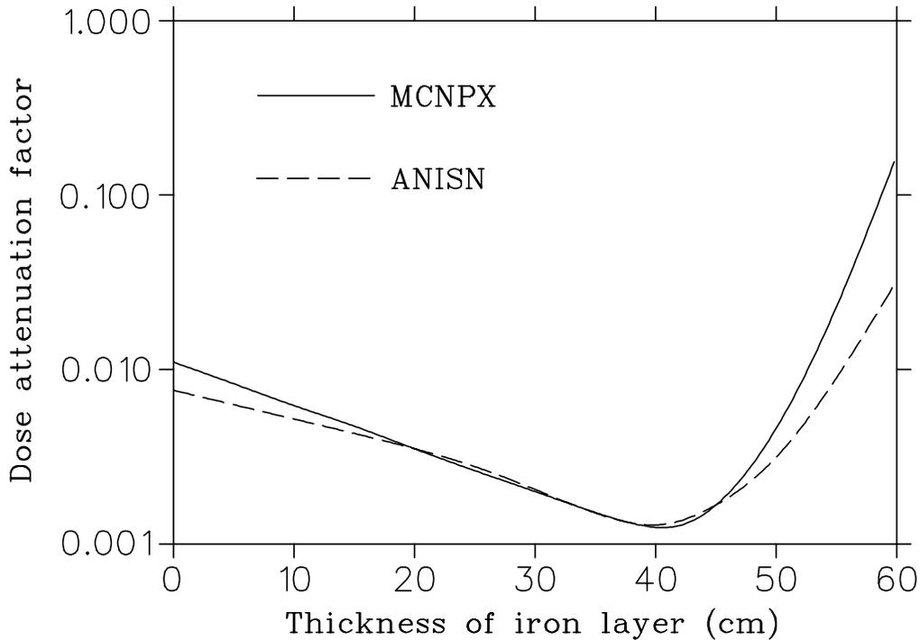
**Figure 2:** Calculated absorbed dose attenuation factors at a point 150 cm from the centre of the Cu target for a 60 cm thick iron/wax spherical shield, plotted as a function of the inner iron layer thickness. The paraffin wax contained 2.5 %  $B_4C$  by weight (see text).
