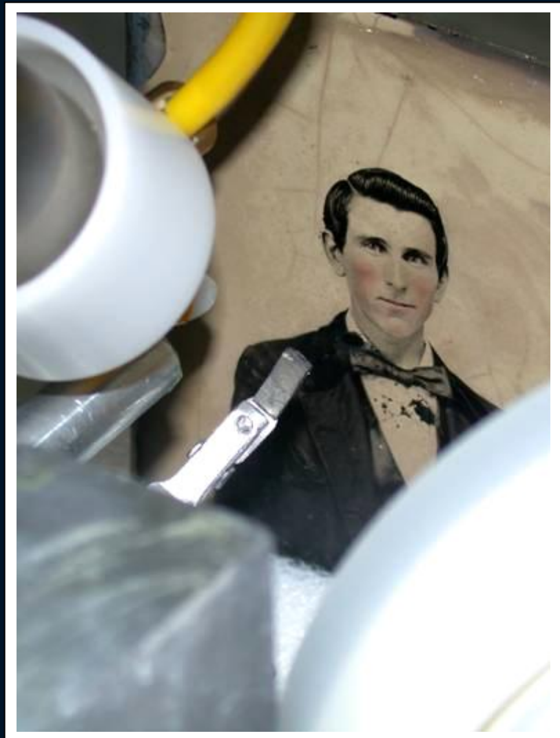
PIXE-PIGE analysis of a print on metal plate of the XIX century
