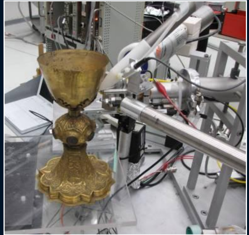
PIXE and PESA analysis of some gilded chalices from the Museum of Casa Siviero, Florence
