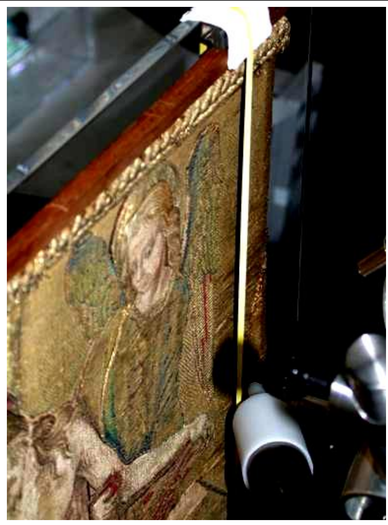
Micro-PIXE and -PIGE analysis of gold threads of a Renaissance embroidery based on a cartoon by Raffaellino del Garbo
