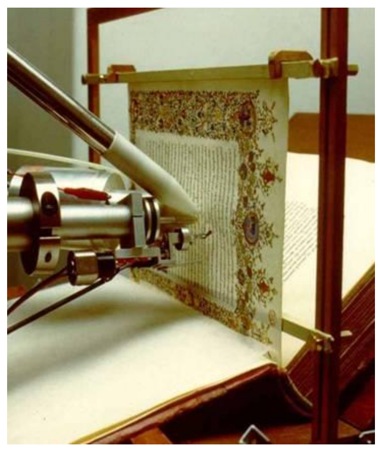
External-beam PIXE analysis of the frontispiece of Pl.16,22 (XV century, Biblioteca Laurenziana in Florence)
