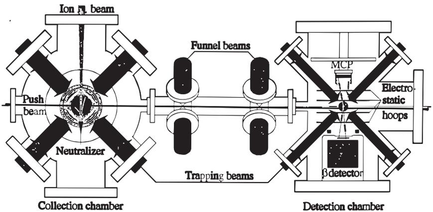
**Fig. 7.** Top view of the TRIUMF two-MOT apparatus. From [69].
