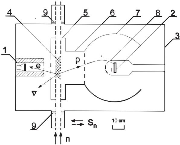
**Fig. 3.** Experimental apparatus used for measuring the  $B$ -parameter in neutron decay. (1) Electron detector, (2) proton detector, (3) vacuum chamber, (4) decay region, (5) cylindrical electrode, (6) TOF chamber, (7) spherical electrode, (8) spherical grid, and (9) LiF diaphragm. From [47].
