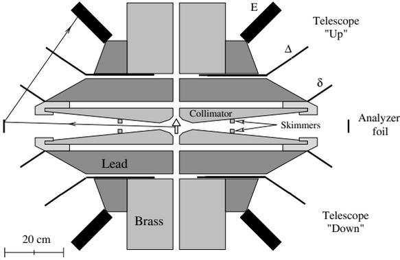
**Fig. 9.** Vertical cross section through the Mott polarimeter used in the  ${}^8\text{Li}$  R-correlation experiment. The direction of incidence of the polarized deuteron beam is perpendicular to the figure. The central arrow indicates the direction of the  ${}^8\text{Li}$  spin in the target. A trajectory of an electron scattered on the lead analyzer foil is also shown. From [93].
